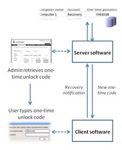
In order to allow recovery into Windows, a similar process is completed. The user dictates a security code to the IT Manager in order to unlock a one-time access code. Upon successful recovery, new codes are generated.
