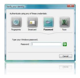
When the user authenticates successfully, the "master encryption key" used to initiate the decryption process is released and used to decrypt the disk. This key is never stored permanently on the hard disk, thus offering a higher level of protection over some file-level encryption solutions.
